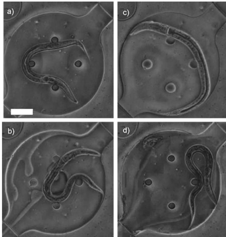
**Fig. 5** Images during device operation: (a) while being cultured on device, animals are suspended in a solution of M9 containing OP50 bacteria; (b) during an imaging cycle, the M9 buffer is first replaced with PF127 solution; (c) the device is then warmed to trigger the sol-gel transition and thus immobilize the worm; (d) after the cycle is complete, the device is allowed to cool off and the PF127 solution is flushed out. Scale bar represents 60  $\mu\text{m}$ .
