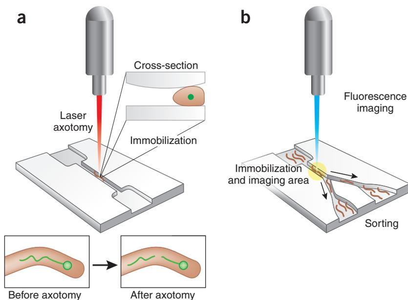
**Figure 1** | Two new applications of microfluidics to study *C. elegans*. (a) Worms are immobilized and positioned for high-resolution axotomy with an ultrafast laser<sup>1</sup>. (b) Worms are sorted at high-throughput based on imaging of desired phenotypes<sup>2</sup>.
